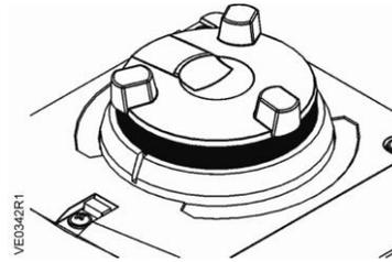
When the motor drives the manual adjuster turns. In Automatic Mode, the manual adjuster is used for indication of travel. If the manual adjuster is held firm in this mode, there is no transmission of power to the gear train.
