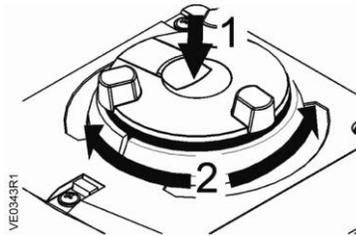
When pushing the manual adjuster down (1), it engages and the actuator can be manually operated.
