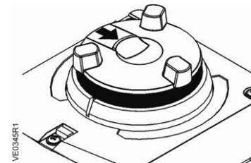
When the black slide switch is pushed back in, and the manual adjuster is not pressed down, the manual adjuster returns to Automatic Mode.
